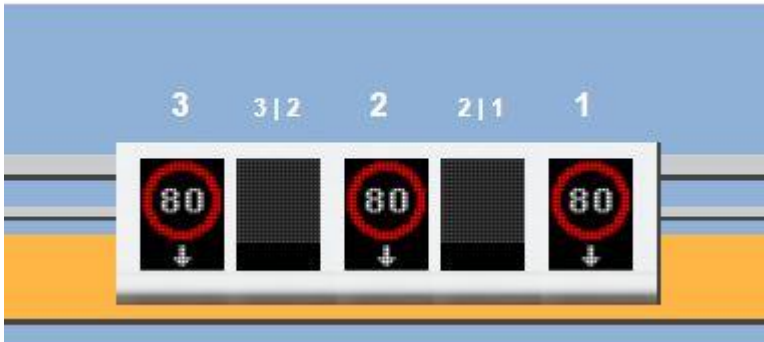
Figure 9b: VMS with lanes specific speed limits
