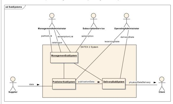
Among the 3 subsystems, DATEX II only describes the delivery subsystem: that means that each developer is free to build:
